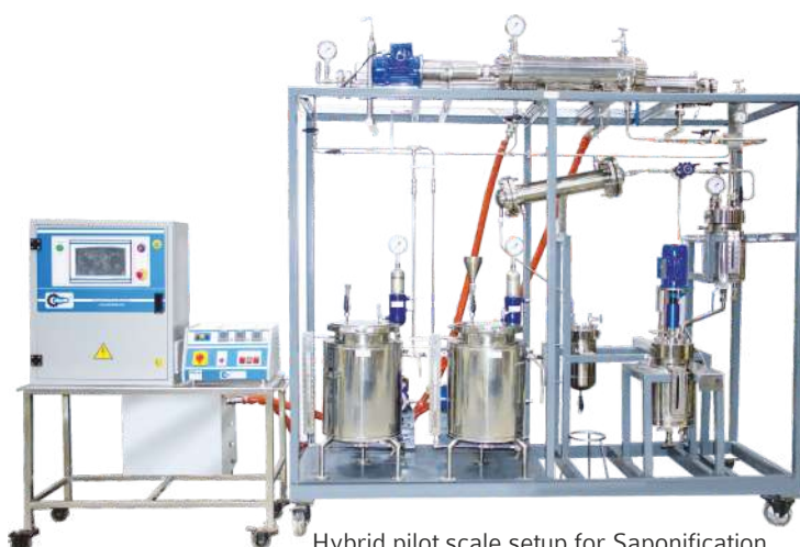
Hybrid pilot scale setup for Saponification using 2.5L VishwaFLO™ & PinchFLO™ reactors
