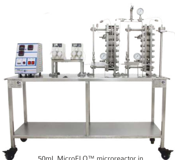
50mL MicroFLO™ microreactor in series (2 nos.) with feed pumps
