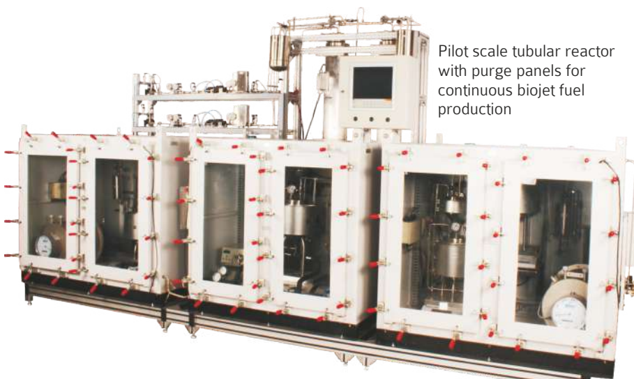
Hybrid pilot scale setup for Saponification using 2.5L VishwaFLO™ & PinchFLO™ reactors
