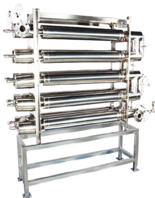
MicroFLO™ + PinchFLO™ for nitration reaction at 10 tons/day
