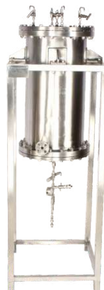
PinchFLO™, 2L Acetylation at 100 LPH
